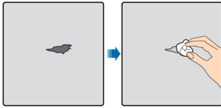
Figure B-2 Treat coating breaks with anhydrous ethanol
